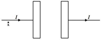
A pair of capacitor plates are charging up due to a current I. The plates have an area A=\pi R^2. Use the Maxwell-Ampere Law to find
