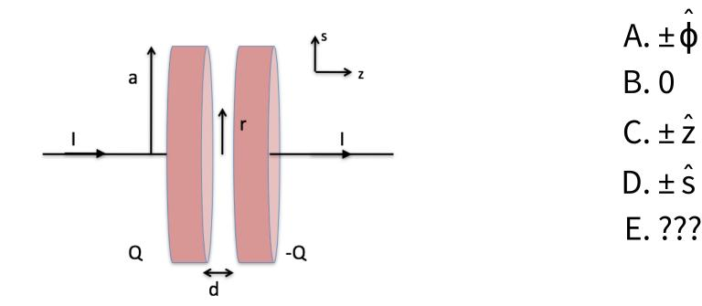
Same capacitor with  $Q = Q_0 + \beta t$  on the positively charged plate. What is the direction of the magnetic field B halfway between the plates, at a radius r?
