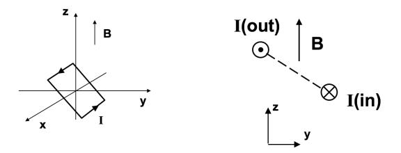
The force on a segment of wire *L* is  $\mathbf{F} = I\mathbf{L} \times \mathbf{B}$  A currentcarrying wire loop is in a constant magnetic field  $\mathbf{B} = B\hat{z}$  as shown. What is the direction of the torque on the loop?
