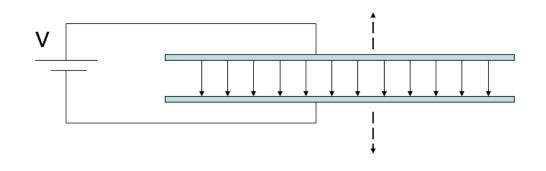
A parallel plate capacitor is attached to a battery which maintains a constant voltage difference V between the capacitor plates. While the battery is attached, the plates are pulled apart. The electrostatic energy stored in the capacitor
